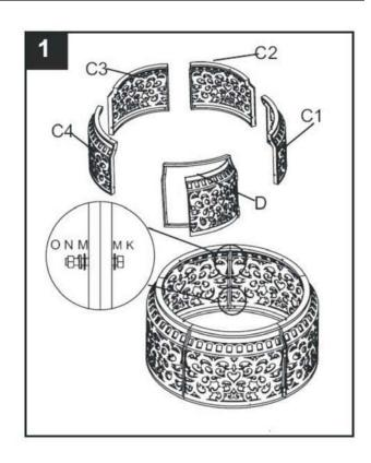
2. Once all Side Panels/Door have been secured, attach Gas Tank Support 1 - H1 to assembled panels by aligning holes in Gas Tank Support 1 with holes in Side Panels/Door. Insert Bolt(6\*32) - K, thru Washer(M6) - M, then insert Bolt/Washer thru holes. Slide Washer(M6) - M over Bolt end, then slide on Spring washer(M6) - N, and secure with Nut(M6) - O. Use Wrench - Q to secure.
