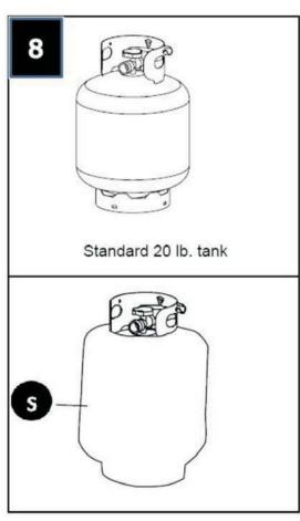
Use the LPG Tank Cover - S to cover the LPG tank prior to placing the LPG tank under the assembled fire pit.
